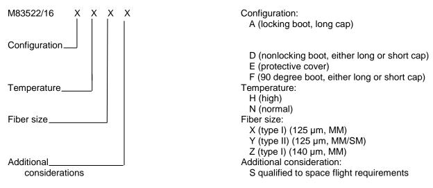
NOTE: Cap refers to the bayonet cap or ST connector outside metal housing. Barrel refers to interior metal part that supports the ferrule and crimp sleeve.
