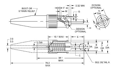
FIGURE 1. Dimensions and configuration.
